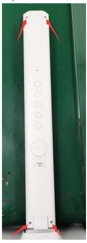
Step8: Pry the shell of lamp-post off directly with the pry piece.
