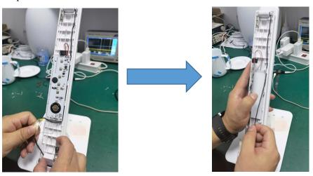
Step11: Pry the shell of lamp hold off directly with the pry piece.
