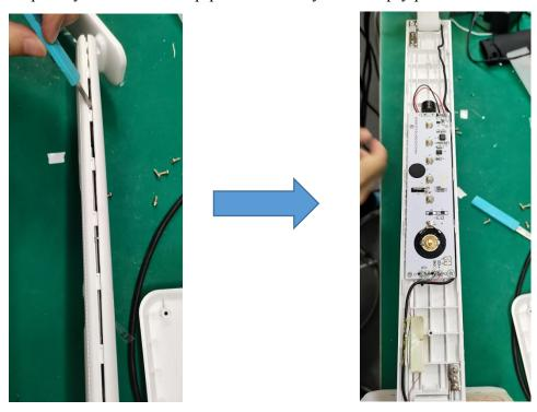
Step9: Remove the 4 screws on Clock PCB board with the screwdriver(PH0x75mm).
