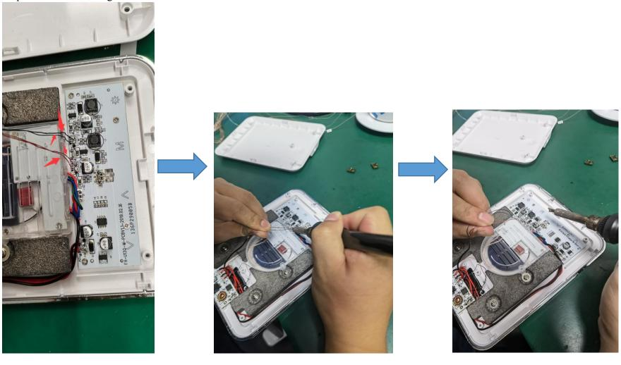
Step5: Remove the 2 screws on DC PCB board with the screwdriver(PH0x75mm).
