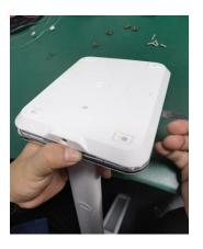
Step3: Pry the shell off directly with the pry piece.
