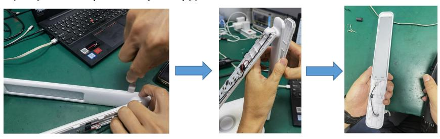
Step12: Remove the 4 screws on lamp holder with the screwdriver(PH0x75mm).
