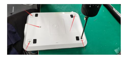
Step2: Remove the 5 screws with the screwdriver(PH0x7 5mm).
