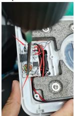
Step6: Straighten the black line and take down the magnetic ring by hand.
