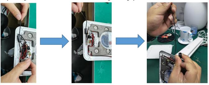
Step7: Remove the 4 screws of lamp-post with the screwdriver(PH0x75mm).
