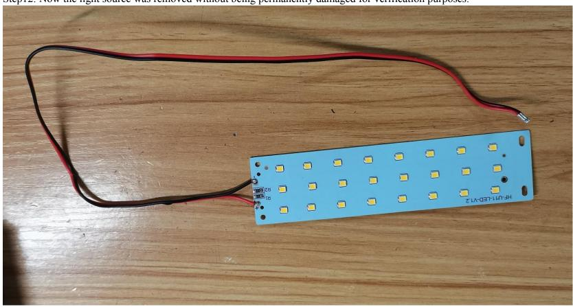
Step12: Now the light source was removed without being permanently damaged for verification purposes.
