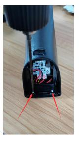
Step3: Remove the 2 screws with the screwdriver(PH0x 75mm).
