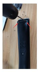
Step4: Remove the 2 screws on lamp-post with the screwdriver(PH0x75mm).
