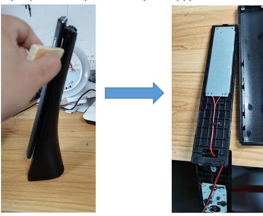
Step10: Remove the 4 screws on LED PCB board with the screwdriver(PH0x75mm).
