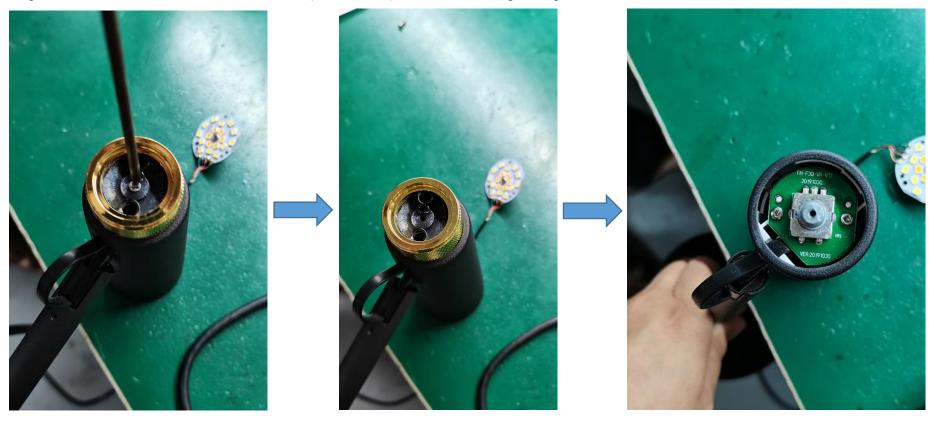
Step4: Remove the 2 screws with the screwdriver(PH0x75mm).
