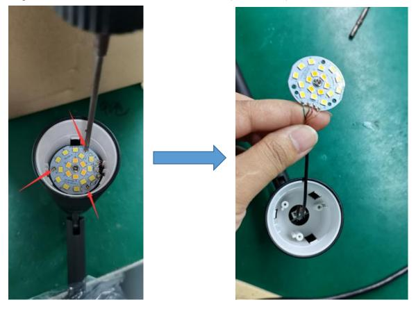
Step3: Remove the screw with the screwdriver(PH0x75mm) then remove the golden part.
