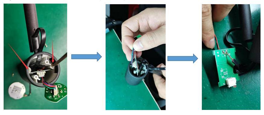
Step6: Use hands to separate the white terminals from the PCB board.
