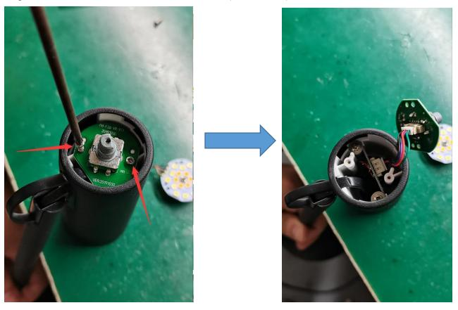
Step5: Remove the 2 screws with the screwdriver(PH0x75mm).
