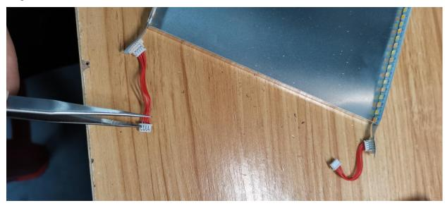
Step5: Now the light source was removed without being permanently damaged for verification purposes.
