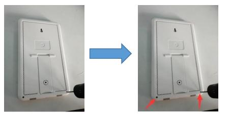
Step2: Pry the shell off directly with the pry piece.
