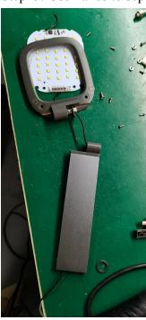
Step16: Bake the pole over a thermal chimney to melt the glue inside, then the part at below arrow is going to come off
