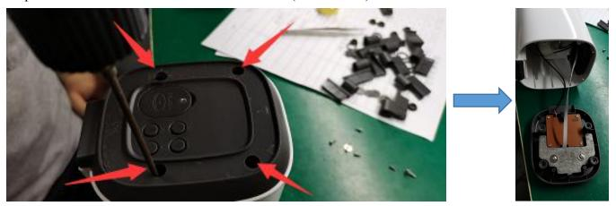
Step3: Remove the 4 screws with the screwdriver(PH0x75mm).
