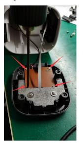
Step4: Use the soldering iron to unsolder the wire from PCB board.
