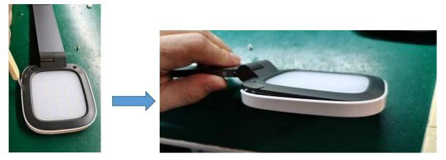
Step9: Remove the 4 screws with the screwdriver.
