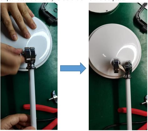
Step4: Remove the 5 screws on lamp holder with the screwdriver(PH0x75mm).
