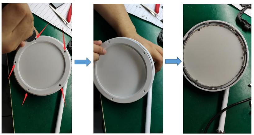
Step5: Pry below part up directly with the pry piece.
