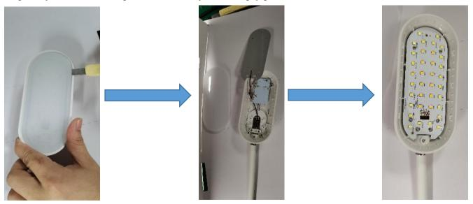
Ste2: Remove the 6 screws with the screwdriver(PH0x75mm).
