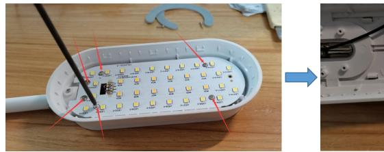
Step3: Use the soldering iron to unsolder.
