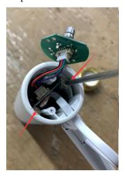
$Step 5: Remove \ the \ screw \ with \ the \ screwdriver (PH0x75mm) \ to \ separate \ the \ inner \& outer \ shell \ of \ lamp \ holder \ .$
