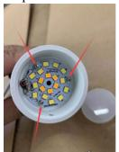
Step9: Use hands to separate the white terminals from the PCB board.
