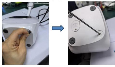
Step2: Use pry piece to pry open along the rear side gap buckle of the fuselage to expose the bottom board.
