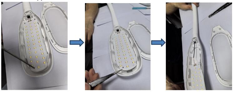
Step7: Now the light source was removed without being permanently damaged for verification purposes.
