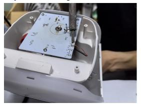
Step4: Use tweezers to pick up the gasket of the lamp head, and then use electric screwdriver to remove the screws of the lamp head.
