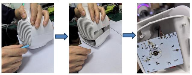
Step3: Use soldering iron to remove the wires from the board.
