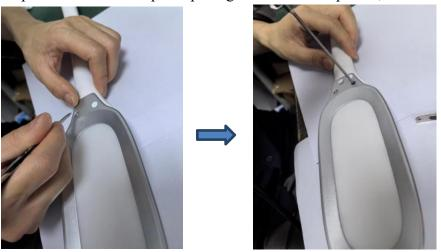
Step5: Use pry piece to pry open along the gap snap of the lamp head.
