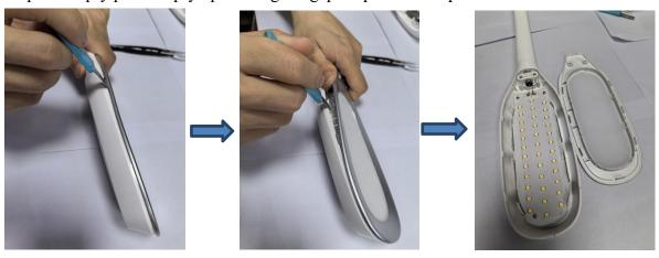
Step6: Use electric screwdriver to remove the screws on the light board, then pick up the light board with tweezer, and pull out the connection wire from the lamp pole.
