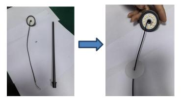
Step7: Use pry piece to lift the light board and separate the light board and the connecting wire from the lamp cap.
