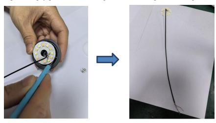
Step8: Now the light source was removed without being permanently damaged for verification purposes.
