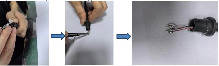
Step5: Use a soldering iron to remove the wires from the connecting plate.
