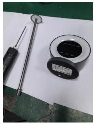
Step2: Fix the lamp cap with one hand and rotate the lamp pole counterclockwise with the other hand at the same time to separate the lamp pole from the lamp cap.
