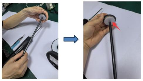
Step3: Use electric screwdriver to remove the screws at the bottom of the lamp pole
