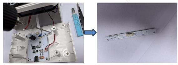
Step5: Now the light source was removed without being permanently damaged for verification purposes.
