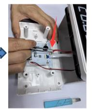
Step4: Use electric screwdriver to remove the screws on the light board.
