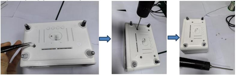
Step2: Use pry piece to pry open with the buckle along the fuselage gap.
