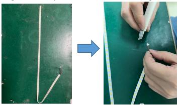
Step7: Now the light source was removed without being permanently damaged for verification purposes.
