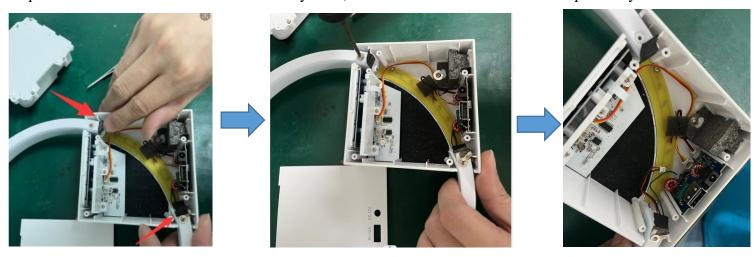
Step4: Then the light pole came out, and then remove the lampshade by hand.
