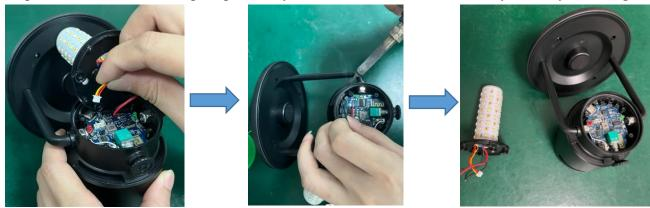
Step5: Remove the screws on the plastic cover of the lighting board with electric screwdriver to separate the plastic cover from lighing board.
