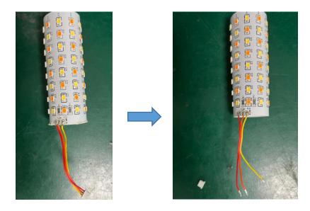
Red line: Positive pole " + " Orange line: Negative pole "-"(cold light) Yellow line: Negative pole "-"(warm light)
