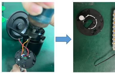
Step6: Use utility knife to raise the wire casing and now the light source was removed without being permanently damaged for verification purposes.
