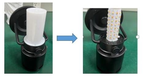
Step3: Remove screws with electric screwdriver and open plastic cover.
