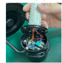
Step4: Remove the wire of lighting board by hand and then remove the battery cable by soldering iron.
